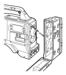
Mount the AU-M402H battery case.
